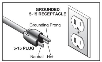
Figure 3. Typical 5-15 plug and receptacle.
